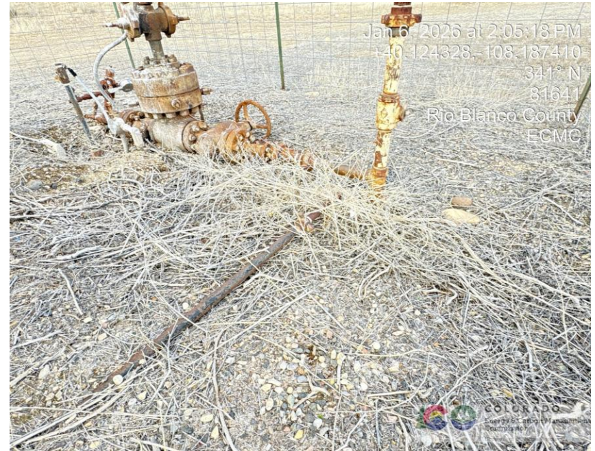
Photo # 0709 Weeds & weed debris near wellhead and pump jack presents a potential fire hazard
