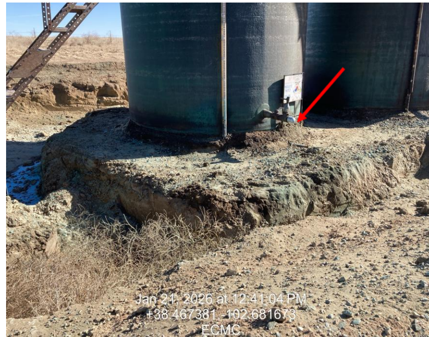
Photo 4 – Impacted soils under tanks
