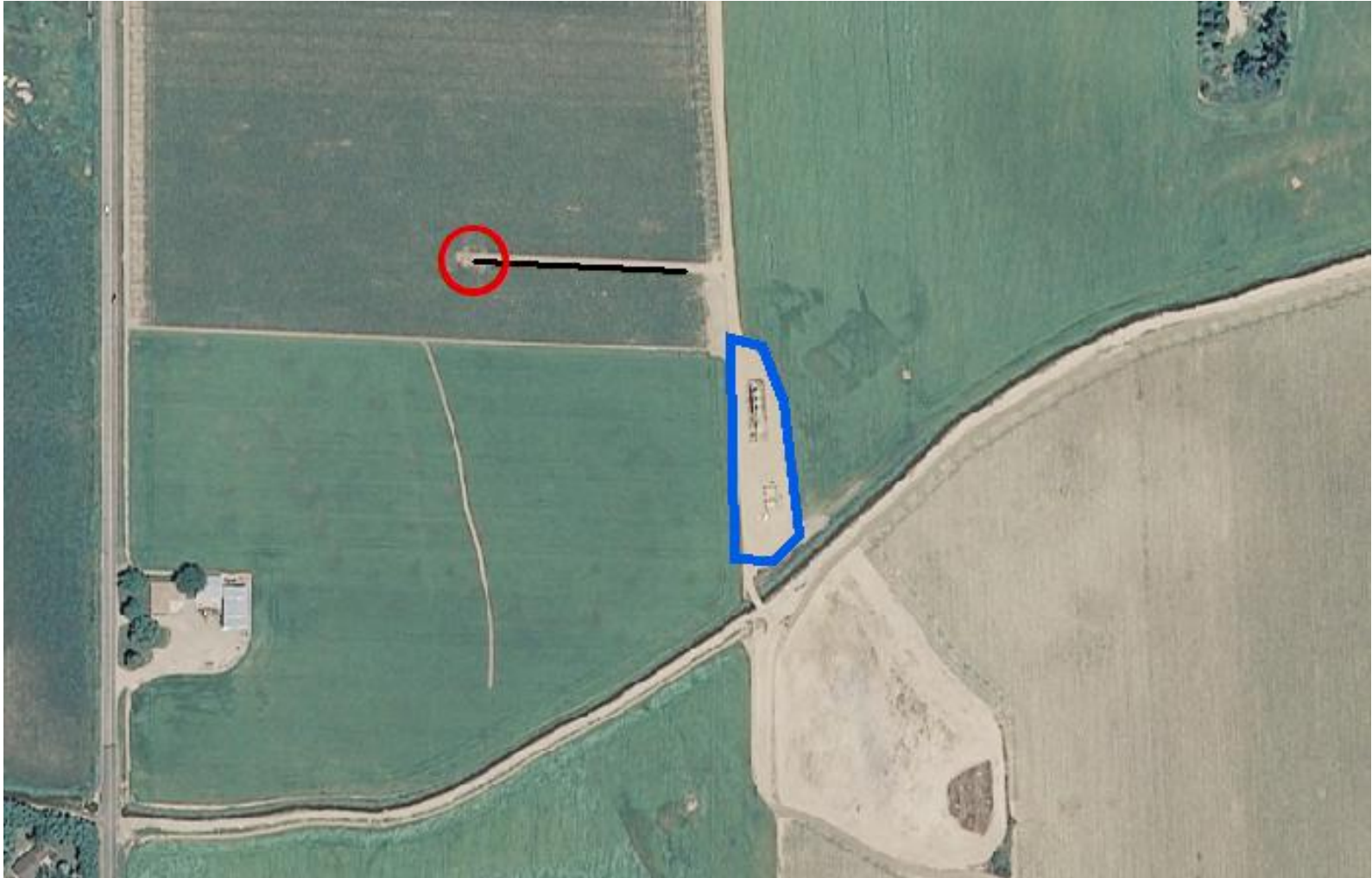
Photo 1. NAIP aerial imagery (2009) illustrating the well location (red circle), associated tank battery location (blue polygon), and well access road (black line). The tank battery is associated with the Bein 6-18 well API #123-25407 under location ID #332702.
