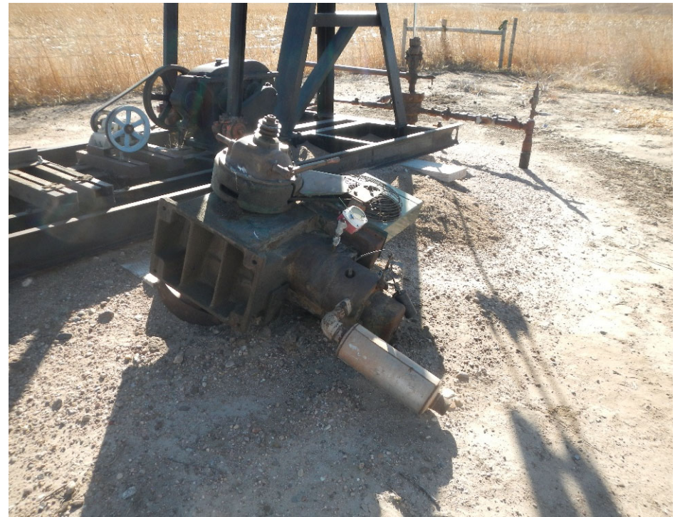
4. Removed prime mover motor inside fencing at well location.
