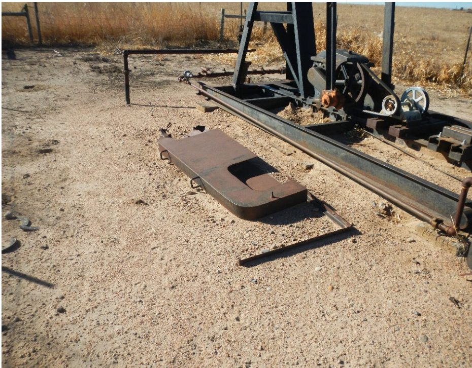
3. Belt guard inside fencing at well location.
