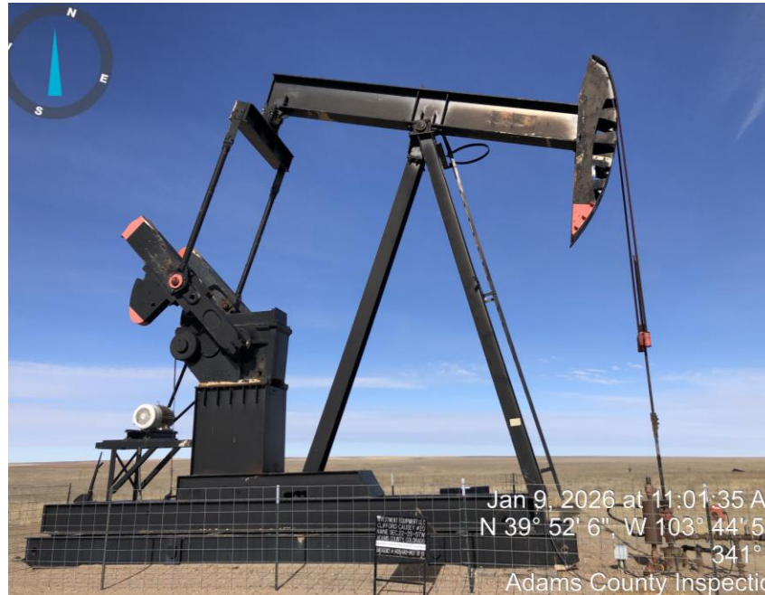
Photo #1 Pump jack.
