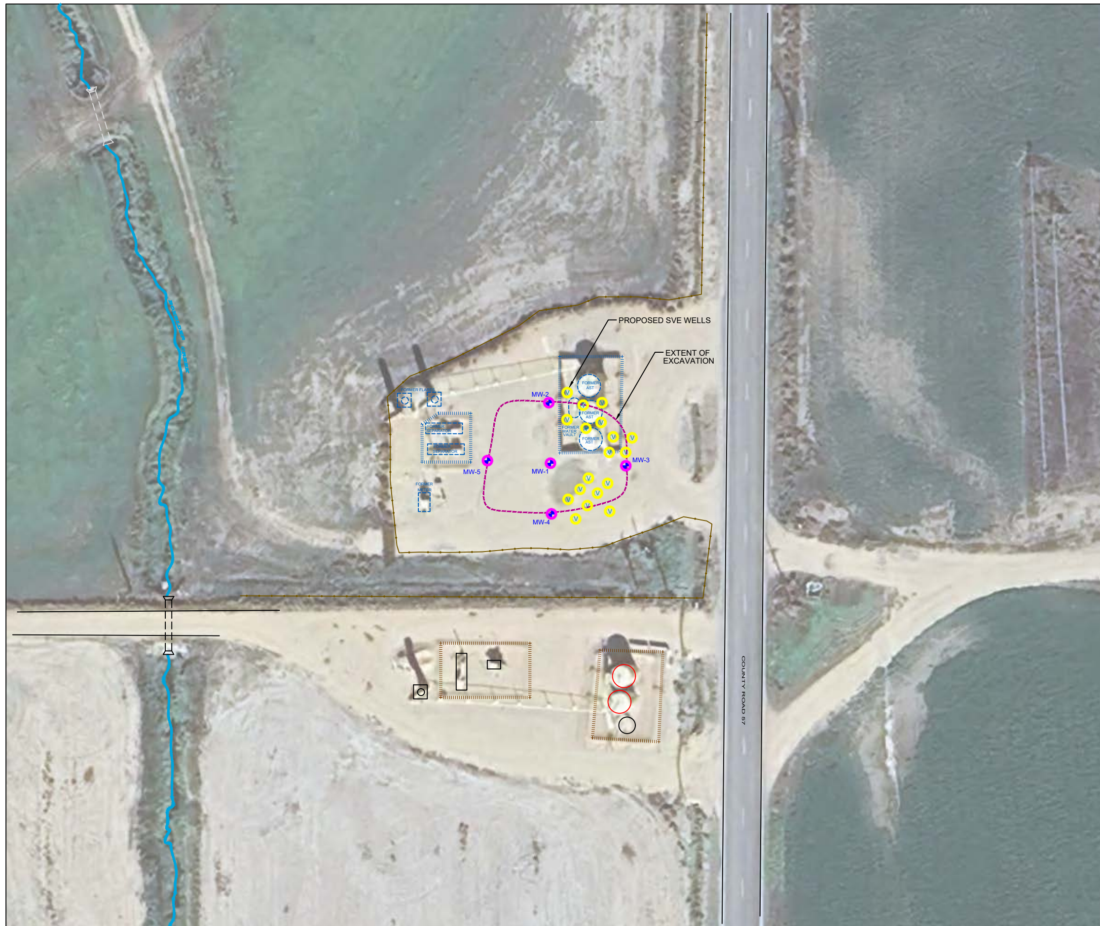
Figure 5 MONITORING WELLS AND PROPOSED SYSTEM WELLS MAP Noble Energy, Inc. Bockius 15-1, 8, Pfannebecker C14-32, D, C, 15-22 SENE Section 15, T4N, R64W, 6th PM Weld County, Colorado 40.312693°, -104.527923°
