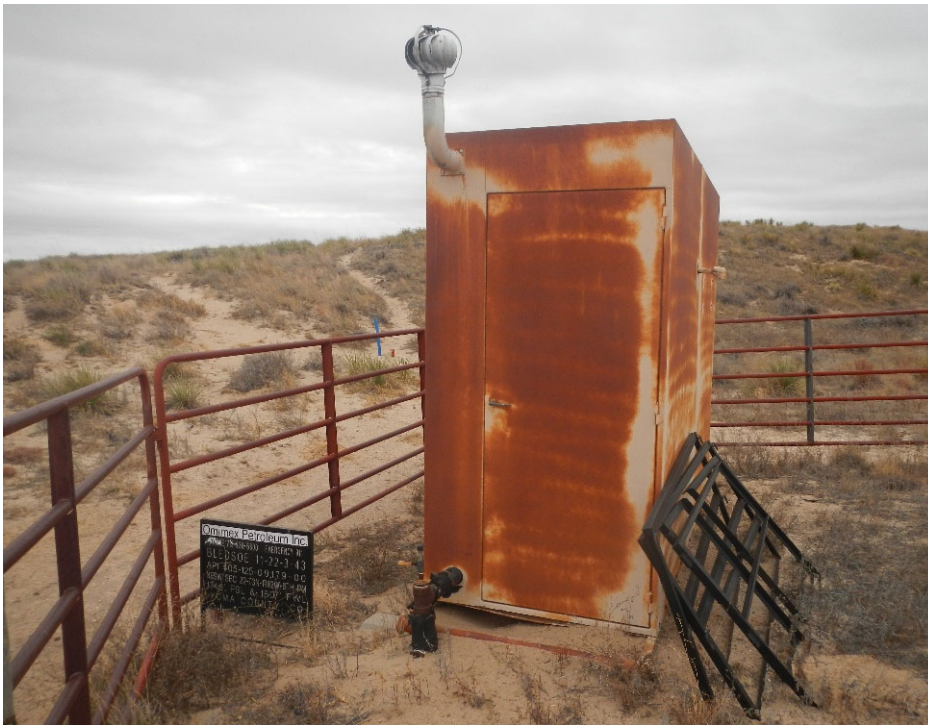
5. Steel separator/meter shed with flowline from well entering shed in lower left corner.
