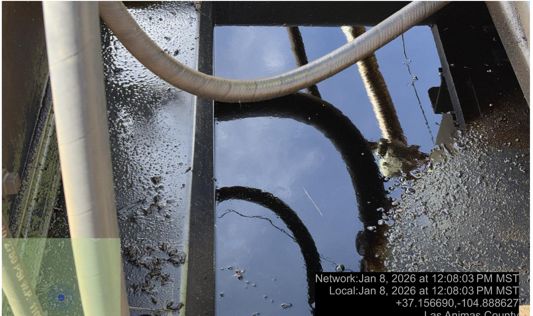
PHOTO 7: There is oily fluids in the engine skid and stained material at the engine exhaust pipe. Conduct maintenance on equipment, cleanup stained material and review self inspection processes. THIS IS THE SECOND NOTICE FOR THIS CA IMMEDIATE ACTION IS REQUIRED.
