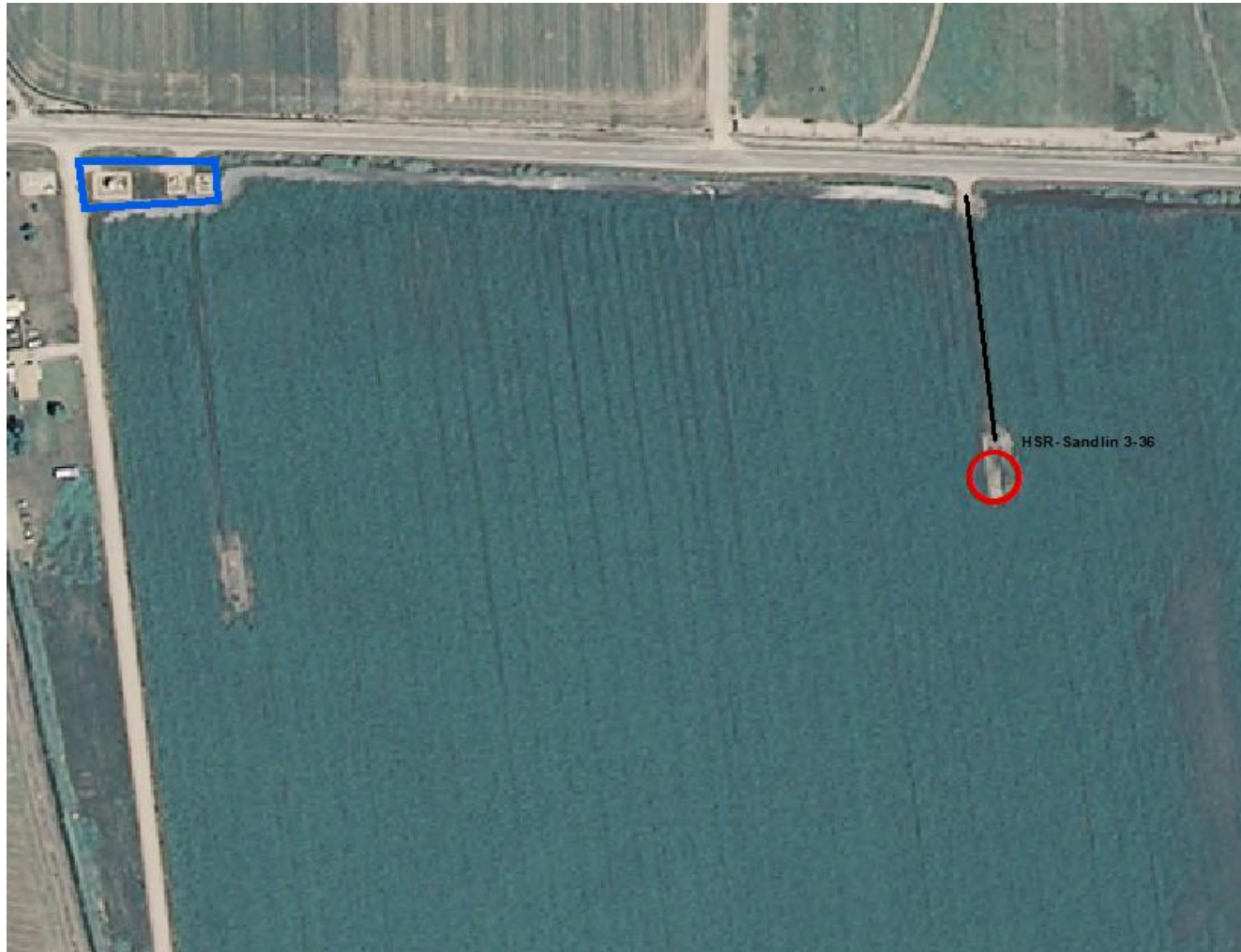
Photo 1. NAIP aerial imagery (2009) illustrating the well location (red circle), associated tank battery location (blue polygon), and access road (black line). The tank battery is associated with its own location ID #445906.
