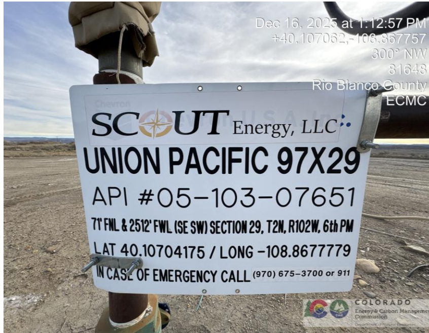
Photo # 0272 Wellhead sign lacks public road used to access the well
