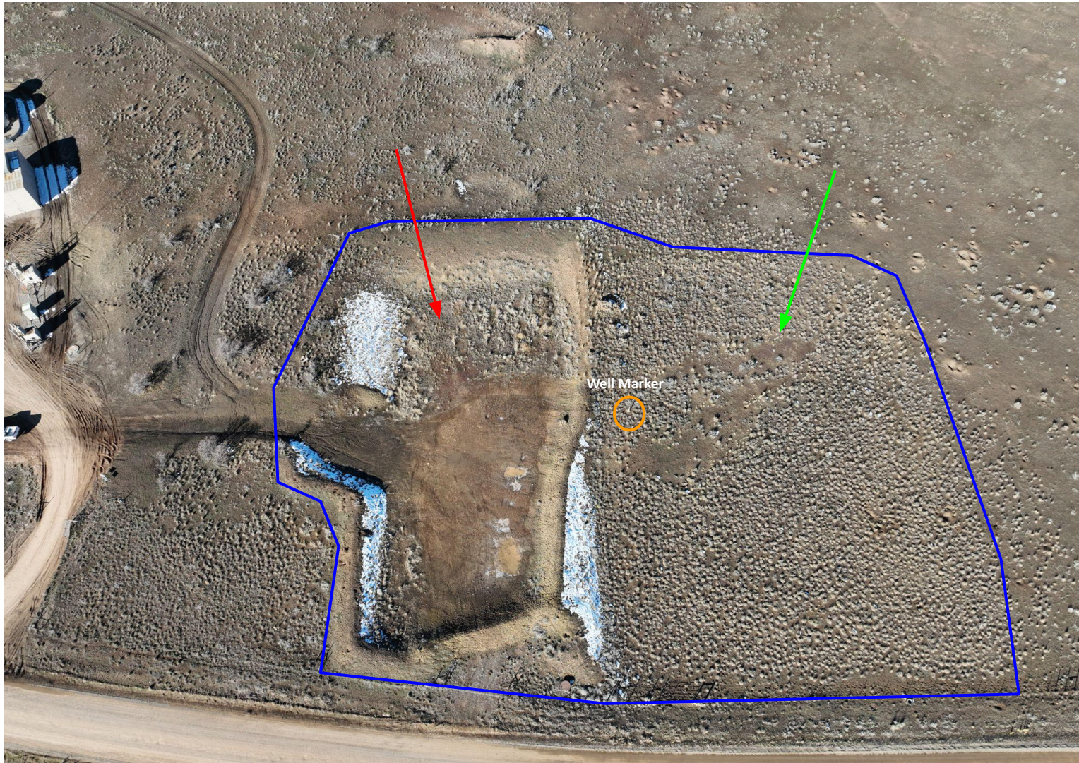
Photo 1. Aerial photo of the location taken with a drone during the time of the inspection from directly above the project area. Note: Entire project area has been outlined in blue. western portion which has not been reclaimed (indicated by red arrow) and Eastern portion of project area which appears to have been reclaimed per 1004 rules and standards (indicated by green arrow).
