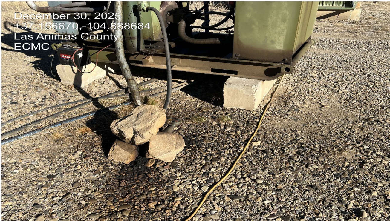
Photo 3. There are stained soils at the exhaust pipe and oily fluids inside the engine skid that need to be cleaned up.
