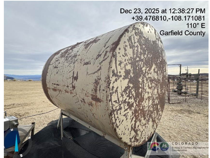
Photo # 5627 Methanol tank lacks required information
