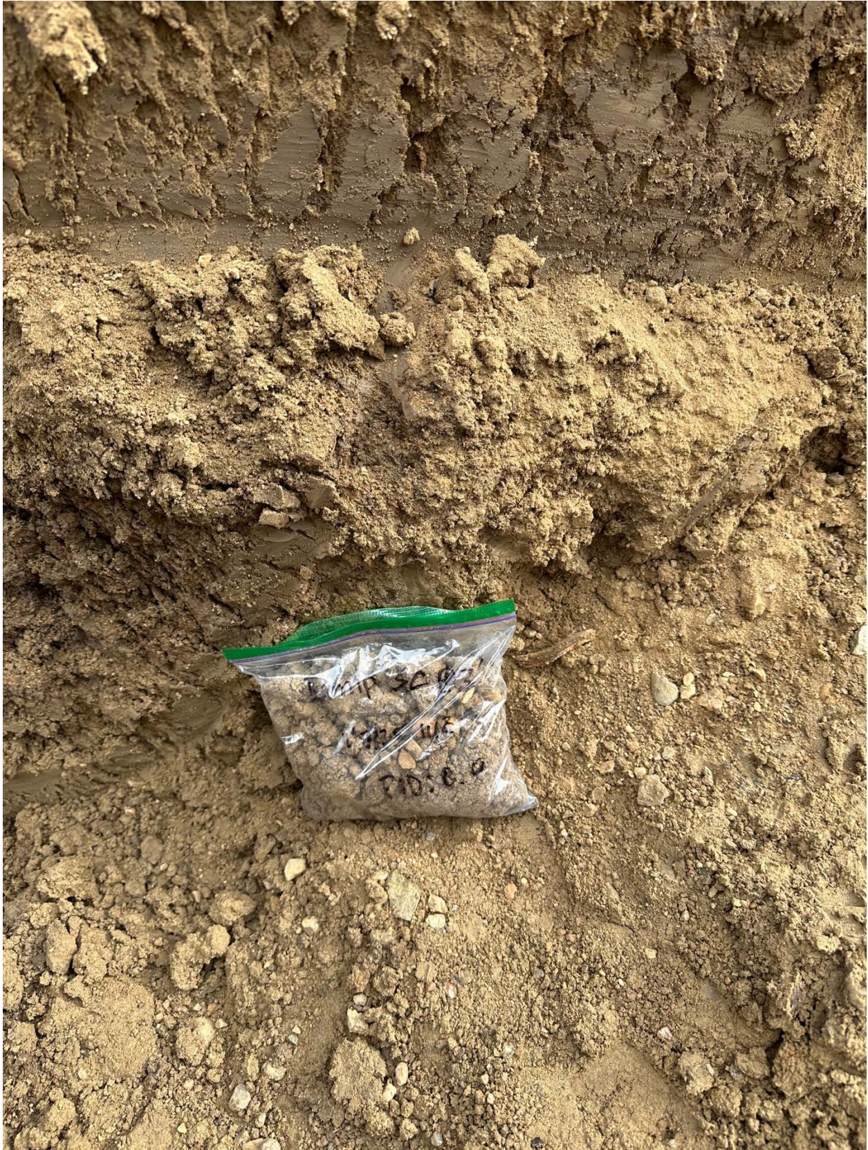
Dumpline Removal Trench - Screening Point: DUMP SCS @ 3' PID: 0.0
