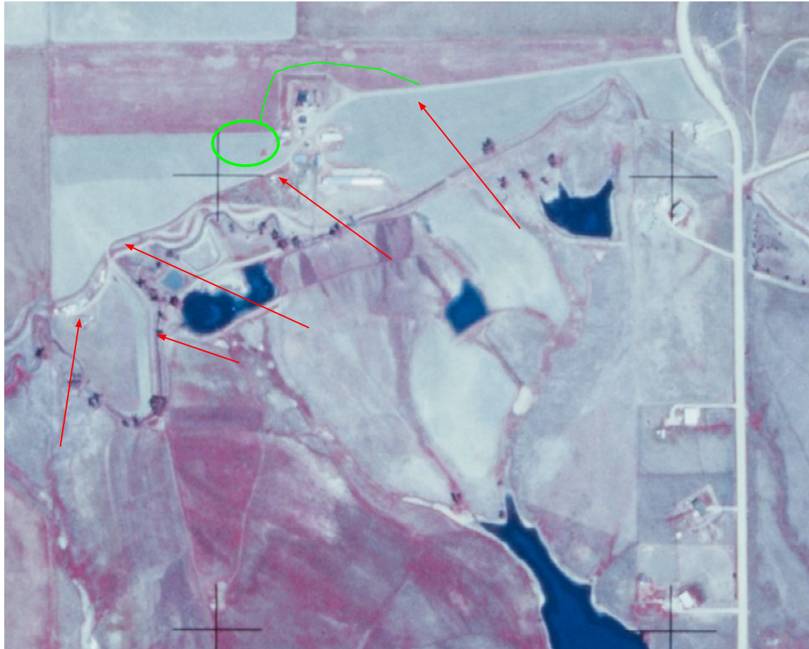
Photo 9. Aerial photograph taken 06-02-1972. The main access road appears to be preexisting to oil and gas development (red arrows). Approximate tank battery access road and location are displayed in green.
