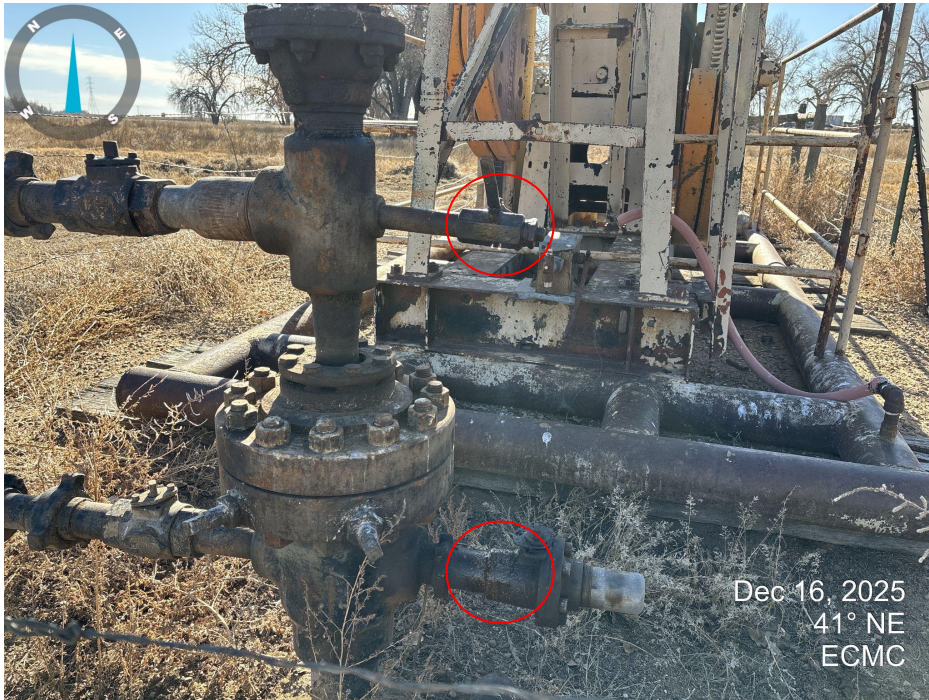
Photo 3. Picture taken at the wellhead. Fluid was visible on the upper valve and beneath the valve.
