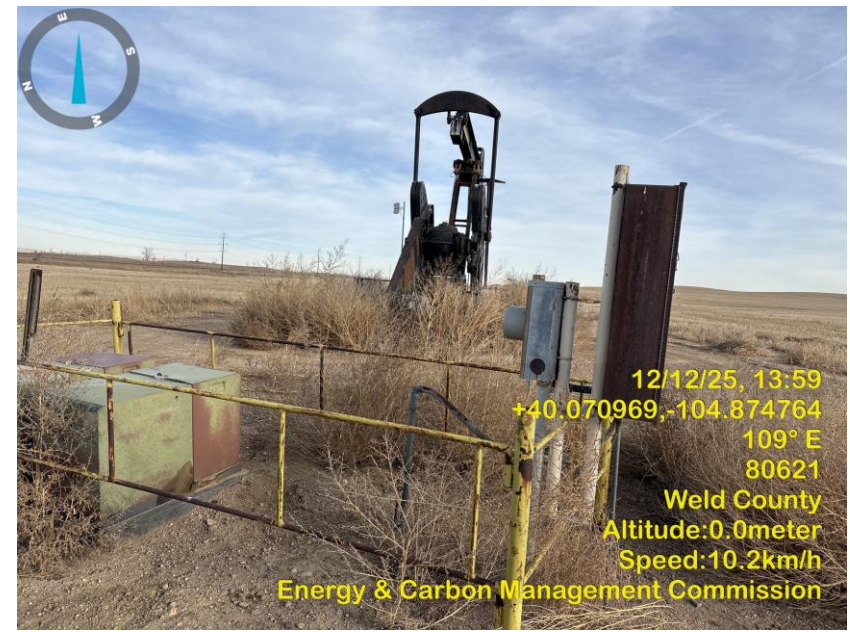
Photo 2 Ancillary equipment overrun with dead vegetation.
