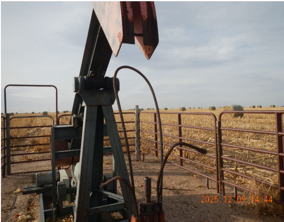
3. Bridle disconnected from Horsehead.
