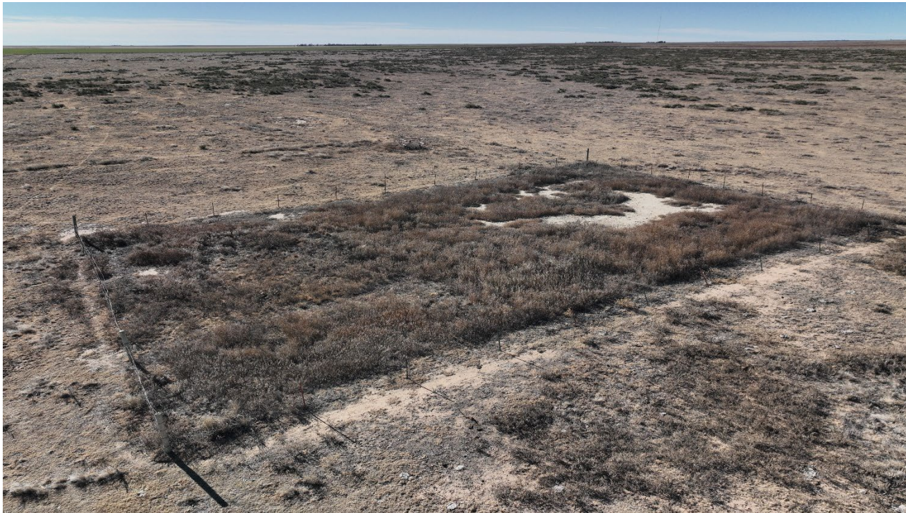
Photo 2. Drone aerial photo facing southwest toward the former wellsite location. The location is fenced but desirable vegetation has not established. The dark vegetation inside the fence is mostly undesirable weeds (Kochia?)
