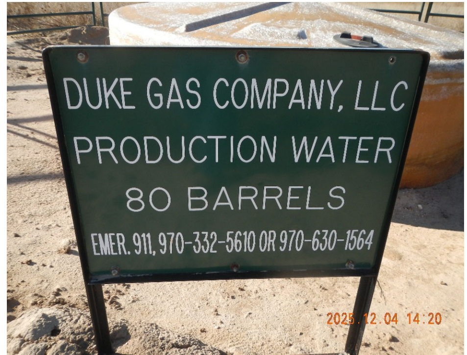
6. Produced water tank sign missing NFPA label.
