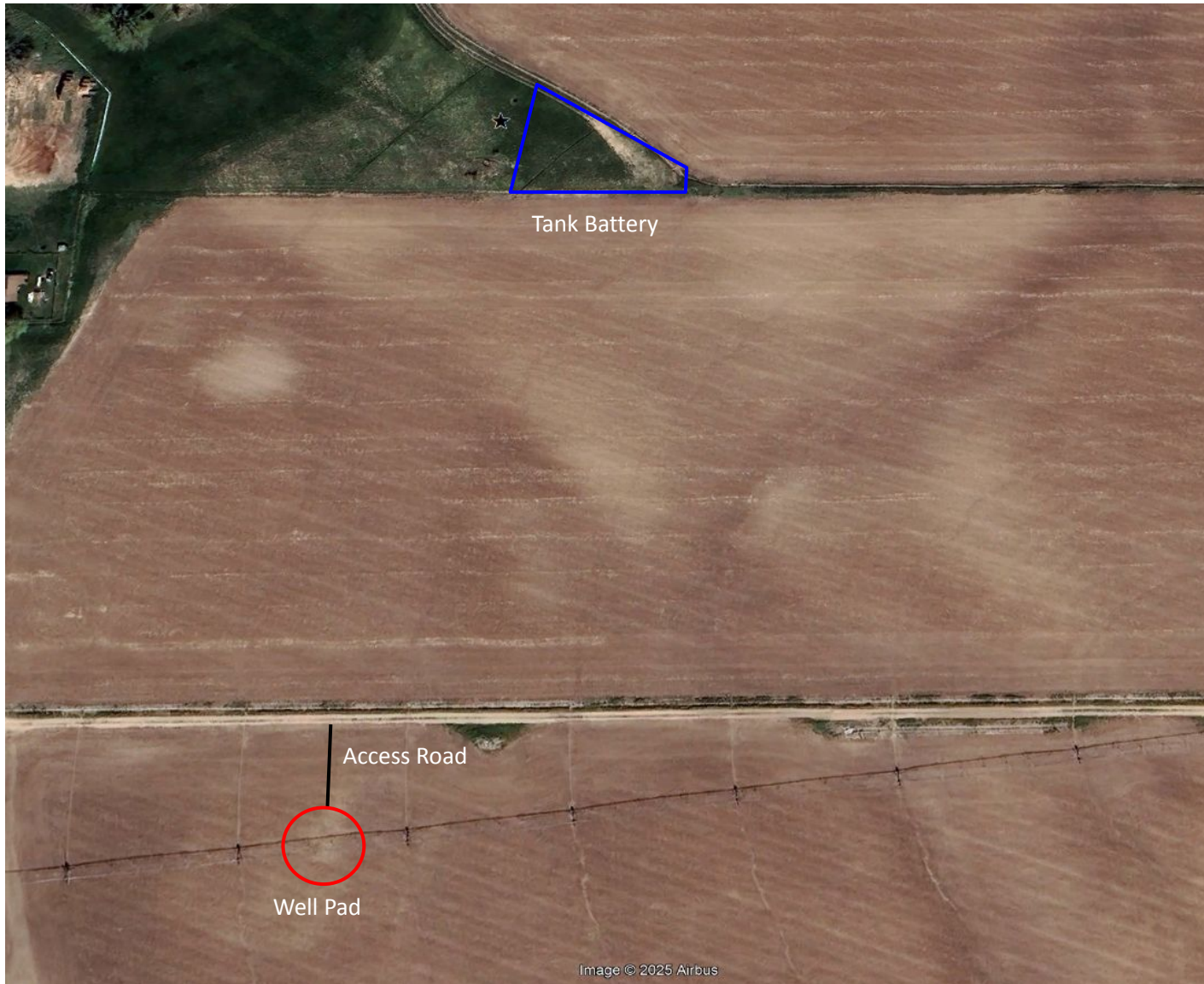
Photo 1. Aerial view of the Well Pad (highlighted in red), Access Road (highlighted in black) and Tank Battery (highlighted in Blue). Note: Tank battery is associated with the Bohlender 1 well API #123-11984 under location ID #322746.
