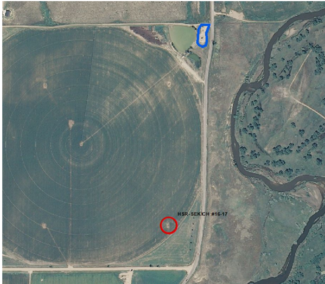
Photo 1. NAIP aerial imagery (2009) illustrating the well location (red circle), associated tank battery location (blue polygon), and well access road. Tank battery is associated with the HSR Sekich 9-17 well API #123-18820 under location ID #330297.
