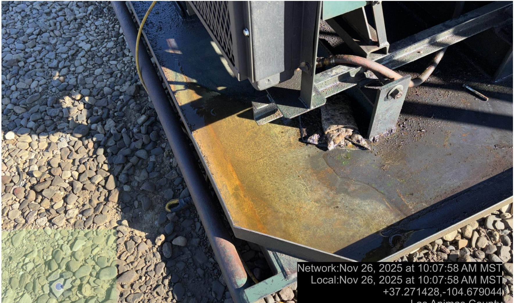
PHOTO 6: OILY WASTE IN COMPRESSOR SKID. DRAIN OILY WASTE REPAIR ALL LEAKS AND REMOVE IMPACTED SOIL PER RULE 1002..(2).D & 1002.f.(2)B, Comply with general provisions of the oil and gas act for wildlife protection AND SB-181. CA DATE 11-27-2025.
