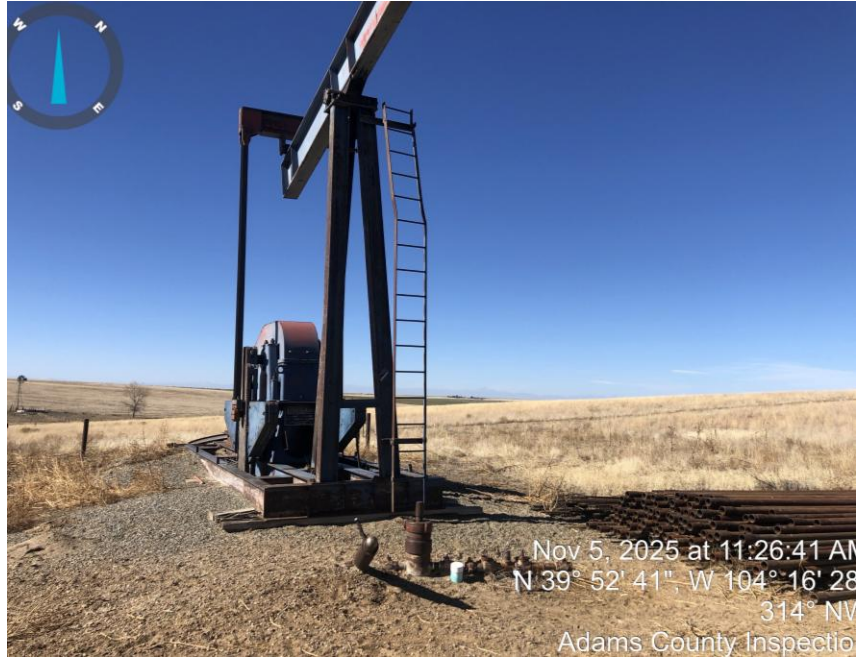
Photo #1 Pump jack & pipe.
