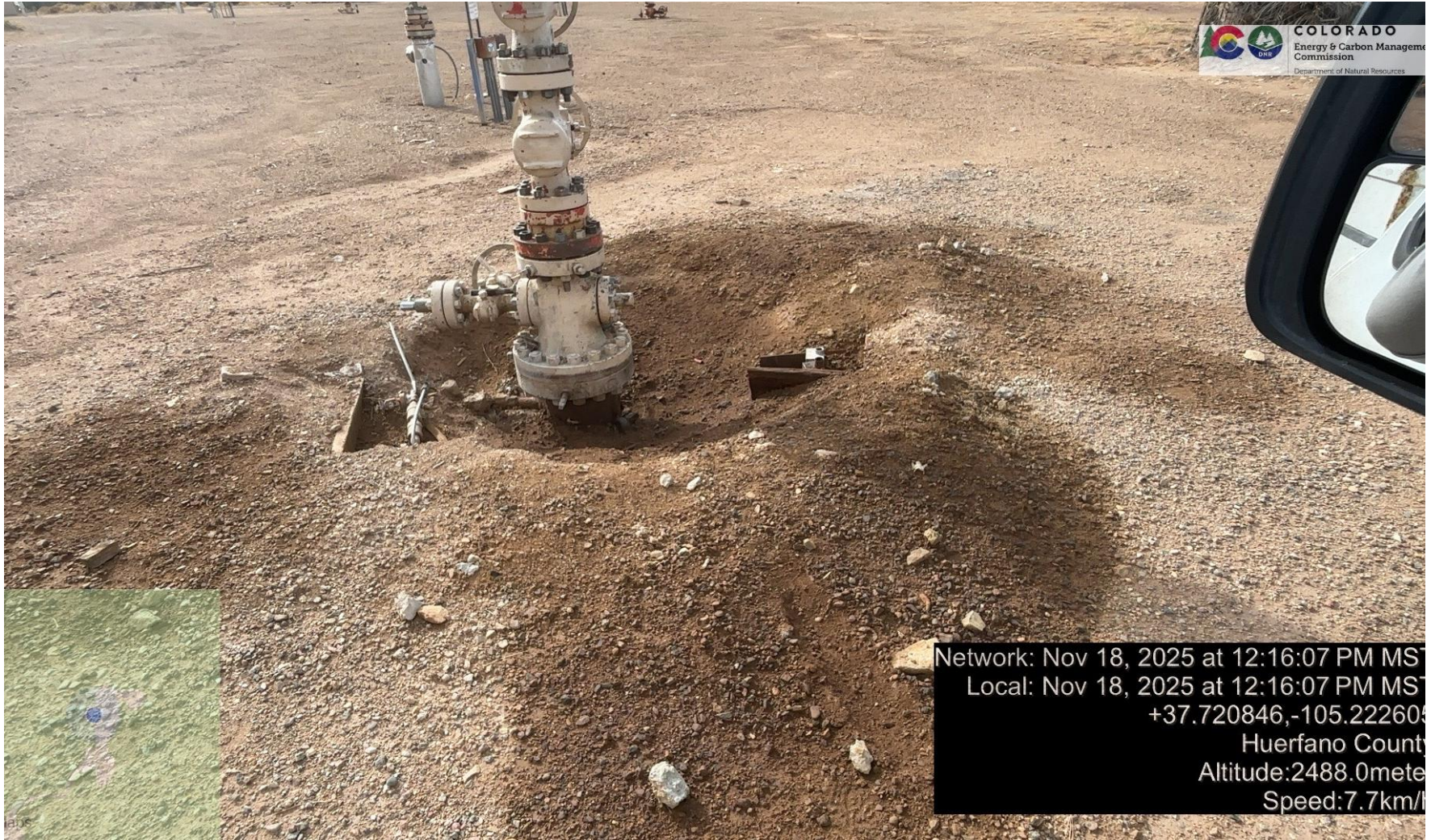
PHOTO 3: AREA OF IMPACTED SOIL AROUND 3-4-0 WELL. Conduct maintenance on equipment, cleanup stained material and review self inspection processes. COMPLY WITH RULE 1002,(2).D
