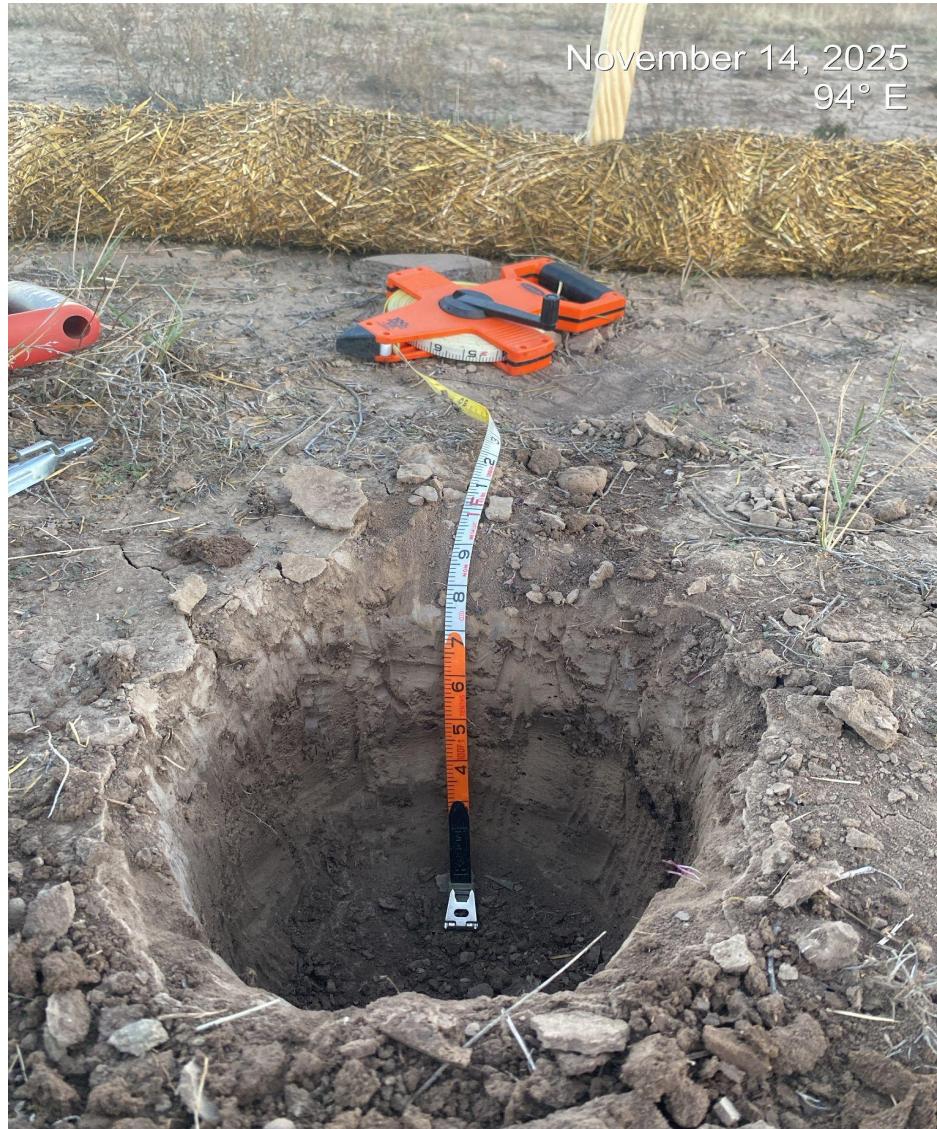
Photo 6. View of soil pit taken in the eastern portion of the disturbance. It was noted that no more than 6 inches of topsoil were observed on site.
