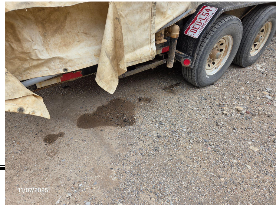
Photo 5: Photos show trailered equipment next to separators/gas lifts. Equipment appears to be leaking resulting in spills onto the WPS.
