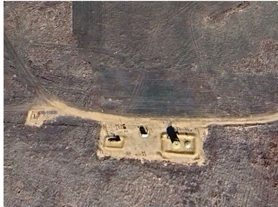
Photo 8. The tank battery to the southeast was reduced when several surrounding wells were plugged. No equipment remains on the closed portion and reclamation has been conducted. The tank battery does not have a separate location ID but is associated with active well API 123-11302.
