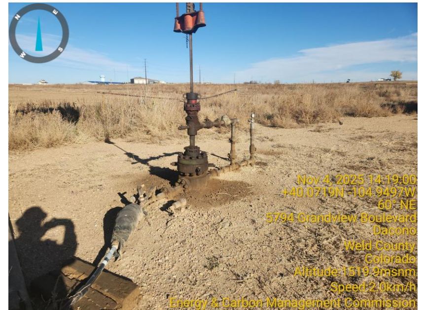
Photo 6 stained soil by the wellhead.
