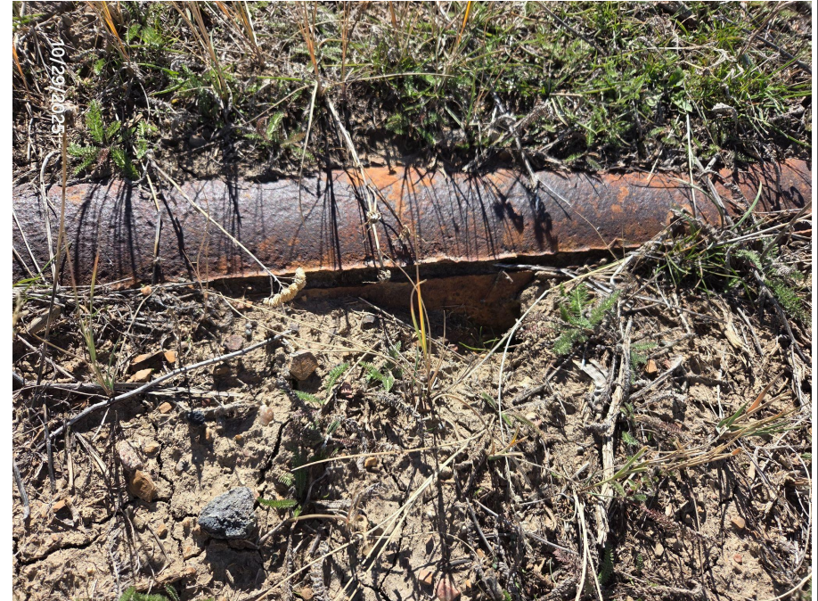
Photo 10: Photos taken from the south end of the Location. Photo shows pipe with a large crack remaining on the Location.
