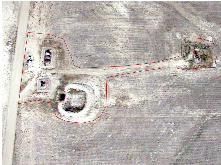
Photo 12. Google earth aerial imagery taken 09/17/2012. Illustrating footprint of the tank battery, access road and well location while active.
