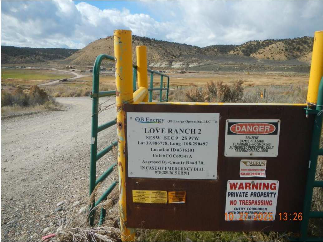
Battery sign is at the gate on CR 5. Not all the information is correct: wrong Location id number (316201) wrong access road (CR20) lat/long not matching wellhead. No api # on sign.
