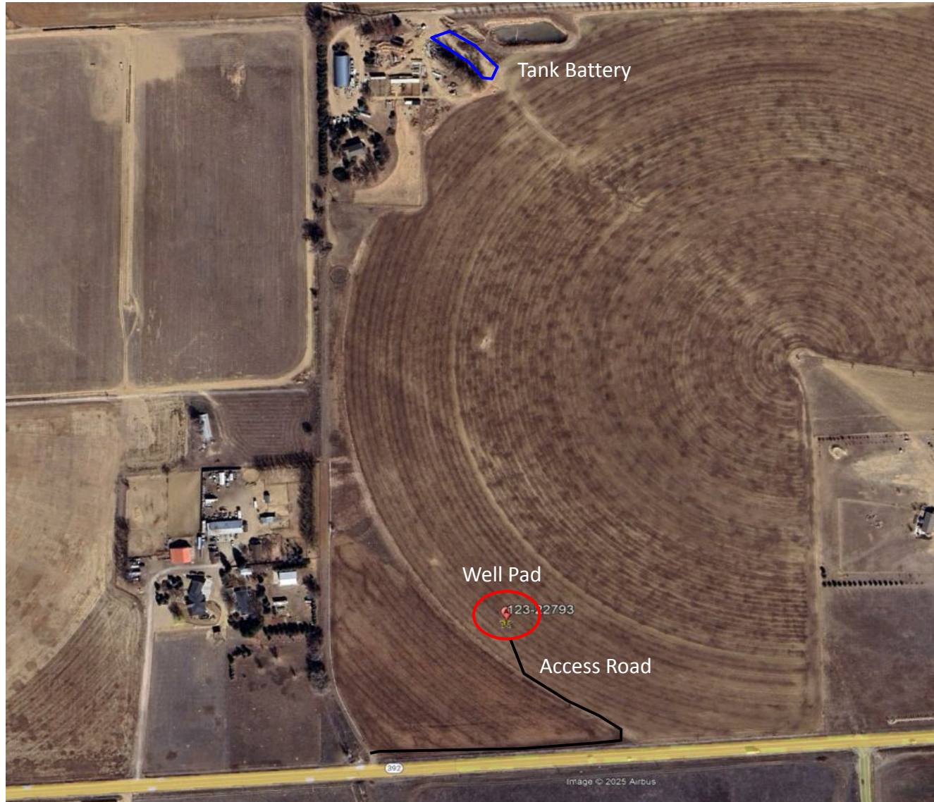
Photo 1. 2025 aerial imagery showing the Tank Battery location (highlighted in blue), Access Road (highlighted black) and Well Pad (highlighted in Red) Note: Tank battery is associated with the Carlson 18-41 well API #123-22792 under the shared location ID #305315.
