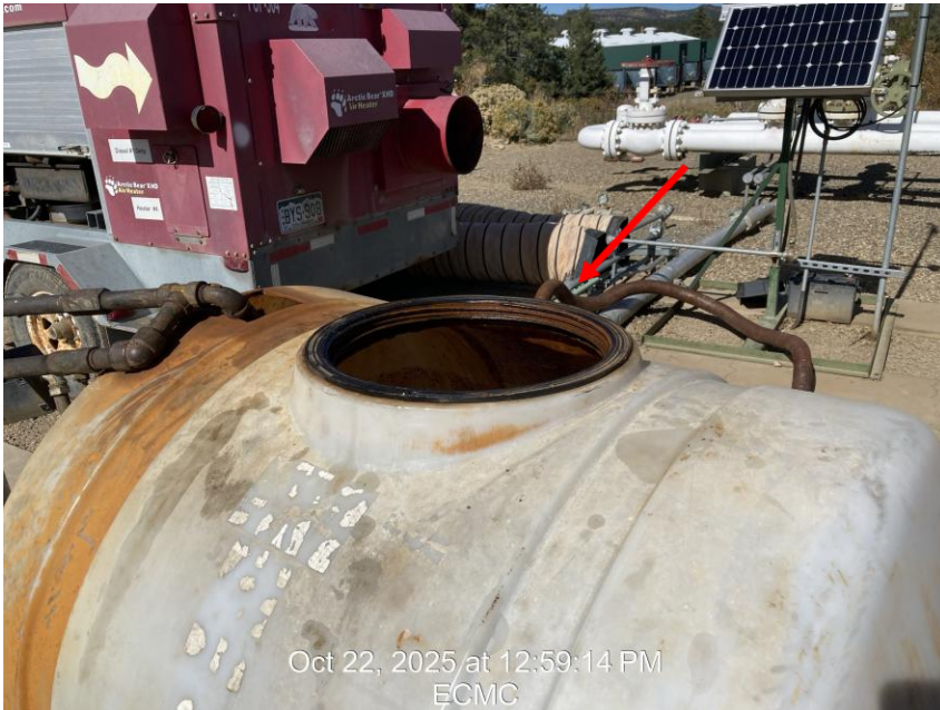
Photo 7 – Missing cap, wildlife protection
