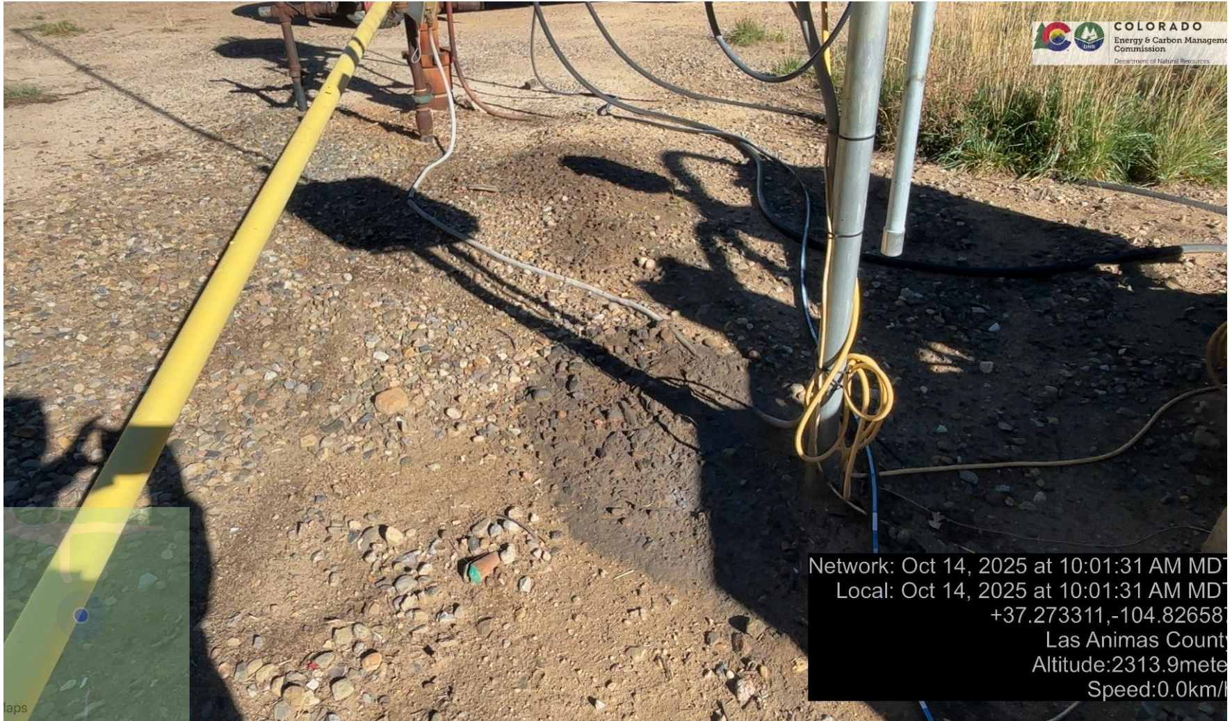
PHOTO 3: AREA OF IMPACTED SOIL BETWEEN WELLHEAD AND PRIME MOVER APPEARS TO BE LEAKING HYDRAULIC HOSE. Conduct maintenance on equipment, cleanup stained material and review self inspection processes. COMPLY WITH RULE 1002,(2).D. CA DATE 11-14-2025.
