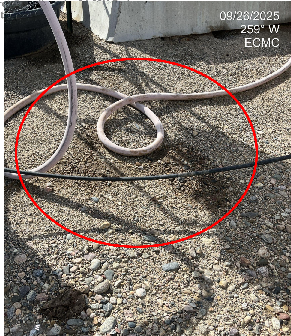
Photo 14. Photos 14-15 taken at the wellhead, illustrating stained soils.
