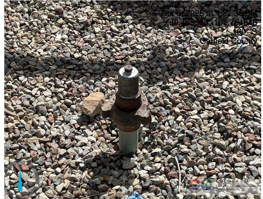
Photo # 4245 Unused flowline lacks lockout tagout (OOSLAT)
