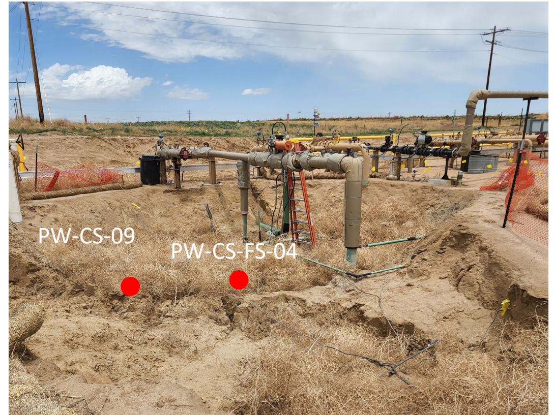
Looking northeast No petroleum hydrocarbon staining or odor observed Visuals limited by tumbleweeds Samples collected: PW-CS-09@8.5' – 1.7 ppm-v PW-CS-FS-04@10' – 1.5 ppm-v
