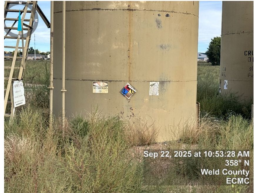
Photo 16: No contents, capacity displayed. NFPA placard damaged
