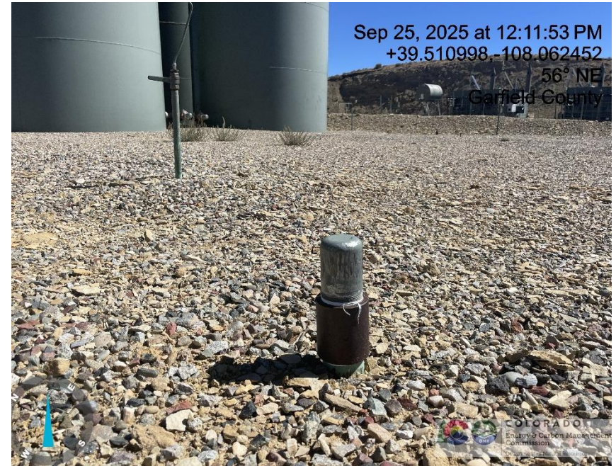
Photo # 2531 Unused flowline lacks lockout tagout (OOSLAT)
