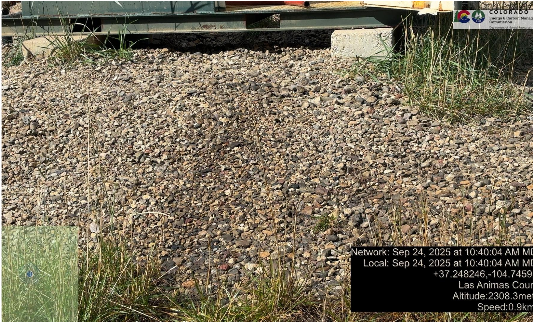
PHOTO 4: AREA OF IMPACTED SOIL OUTSIDE OF SEPARATOR HOUSE APPEARS TO BE FROM DRAINING SEPARATOR ON THE GROUND. IMMEDIATELY DISCONTINUE DRAINING OILY WATER FROM SEPARATOR INTO LOCATION AND Conduct maintenance on equipment, cleanup stained material and review self inspection processes. COMPLY WITH RULE 1002,.(2).D. CA DATE 10-24-2025.
