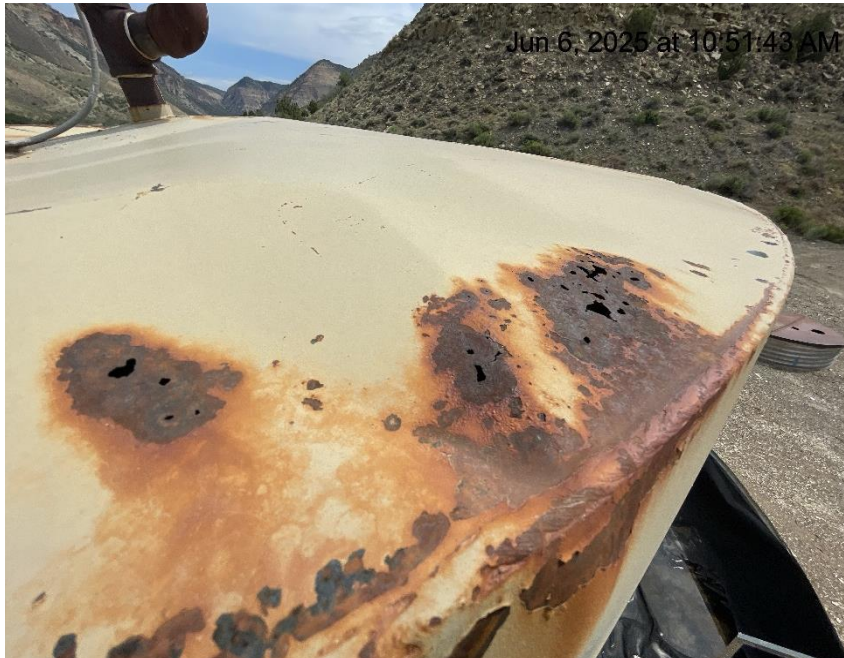
Photo # 6904 From inspection/audit 708906677 conducted on 06/06/2025 Tank failure Multiple holes in tank/tank lacks integrity
