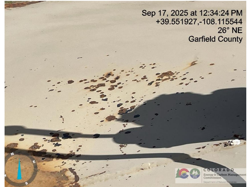
Photo # 284 Tank failure Multiple holes in tank/tank lacks integrity
