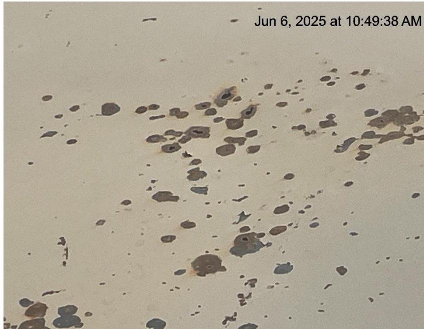
Photo # 6906 From inspection/audit 708906677 conducted on 06/06/2025 Tank failure Multiple holes in tank/tank lacks integrity
