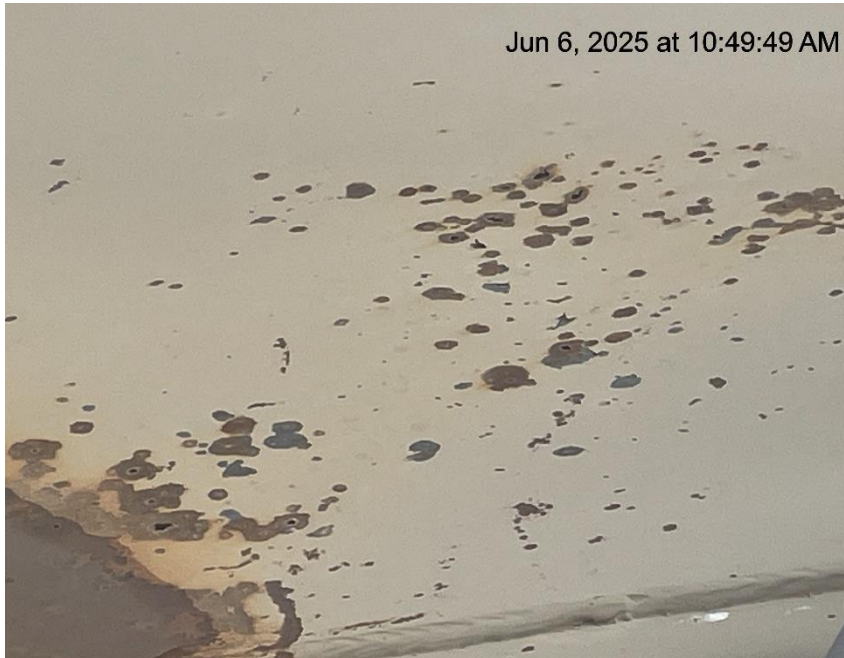
Photo # 6905 From inspection/audit 708906677 conducted on 06/06/2025 Tank failure Multiple holes in tank/tank lacks integrity
