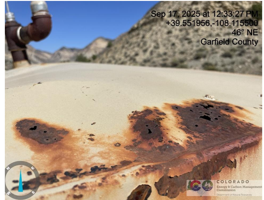
Photo # 283 Tank failure Multiple holes in tank/tank lacks integrity
