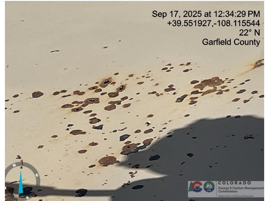
Photo # 285 Tank failure Multiple holes in tank/tank lacks integrity
