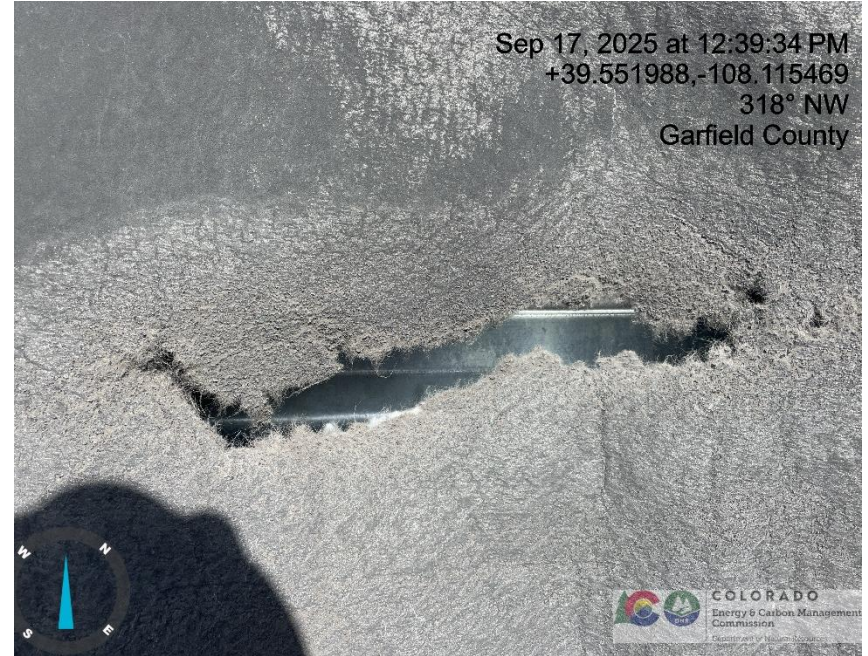
Photo # 288 Hole in liner/liner needs maintenance
