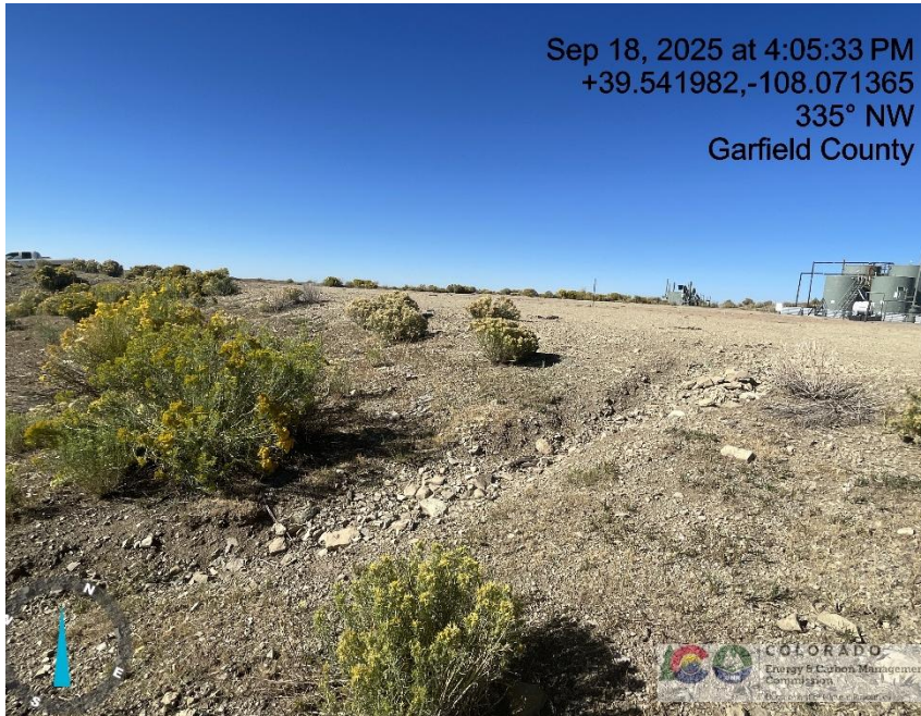
Photo # 1216 Erosion & transport of sediment off location /insufficient BMP's
