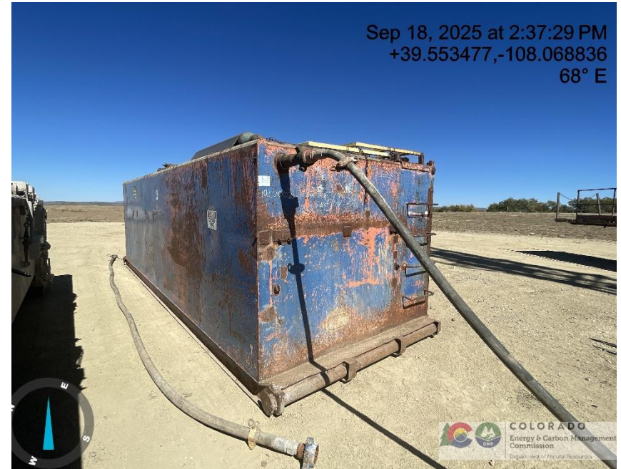
Photo # 1161 Rig tank lacks required labeling
