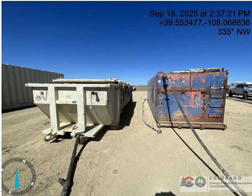
Photo # 1160 Rig tank lacks required labeling
