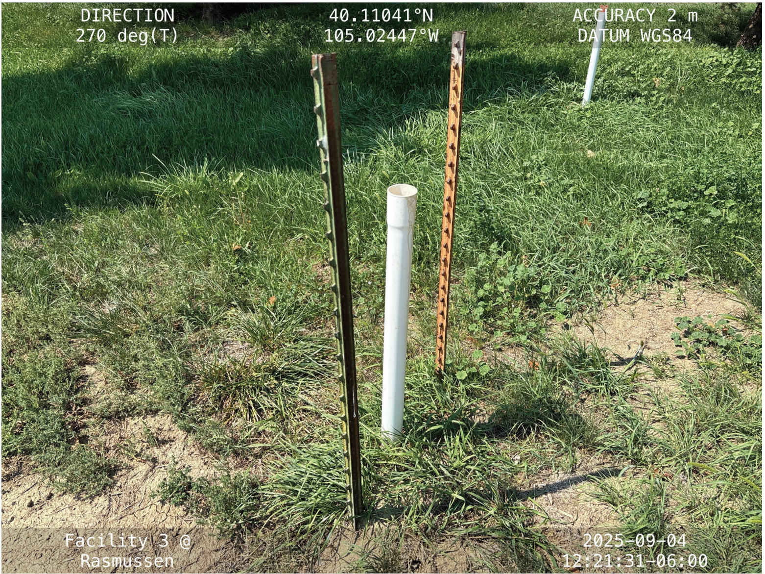
PVC stickup associated with irrigation system - Not a monitoring well.
