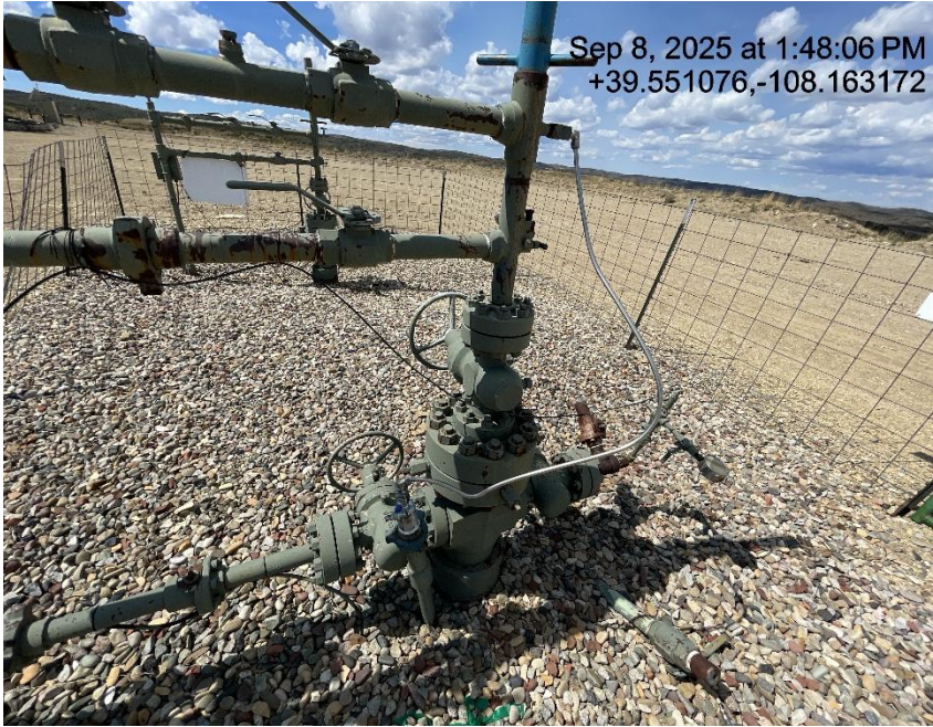
Photo # 6646 CHEVRON 275-1 BH line tied into flowline/no FORM 4 SUNDRY & no check valve
