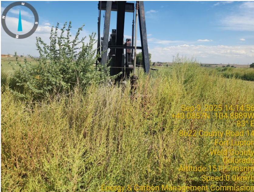
Photo 9 Wellhead is overrun with vegetation .
