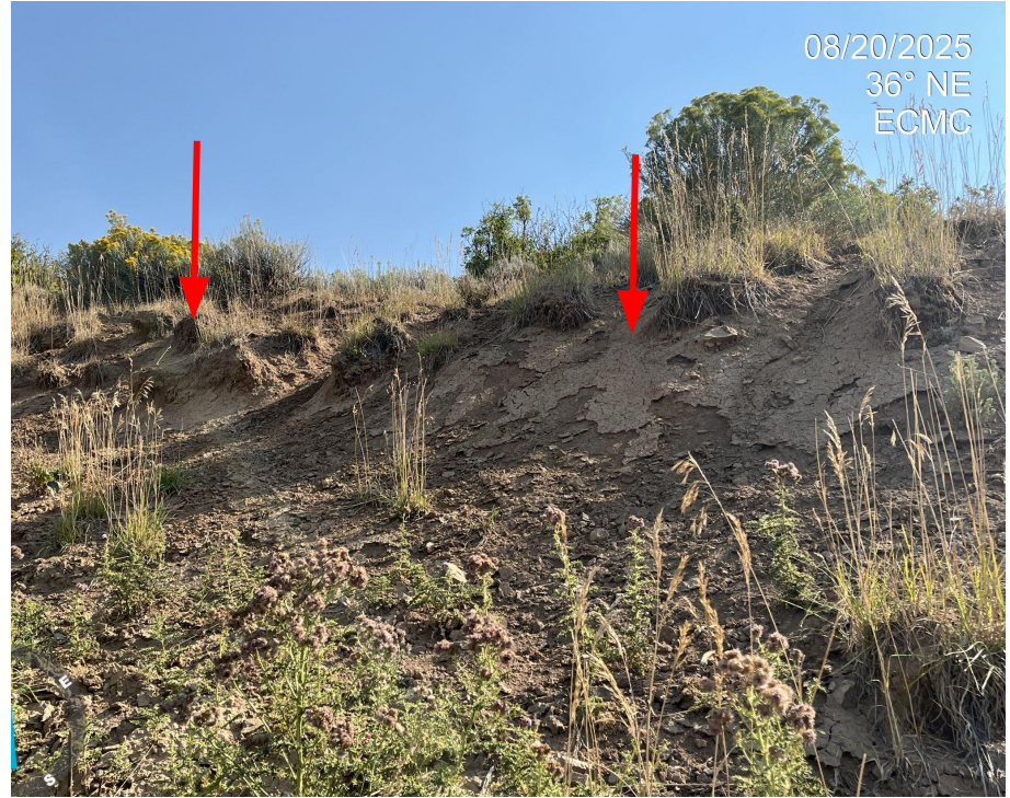
Photo 8. See comments under Photo 6. Red arrows point to bare slopes and where erosion has started to occur.
