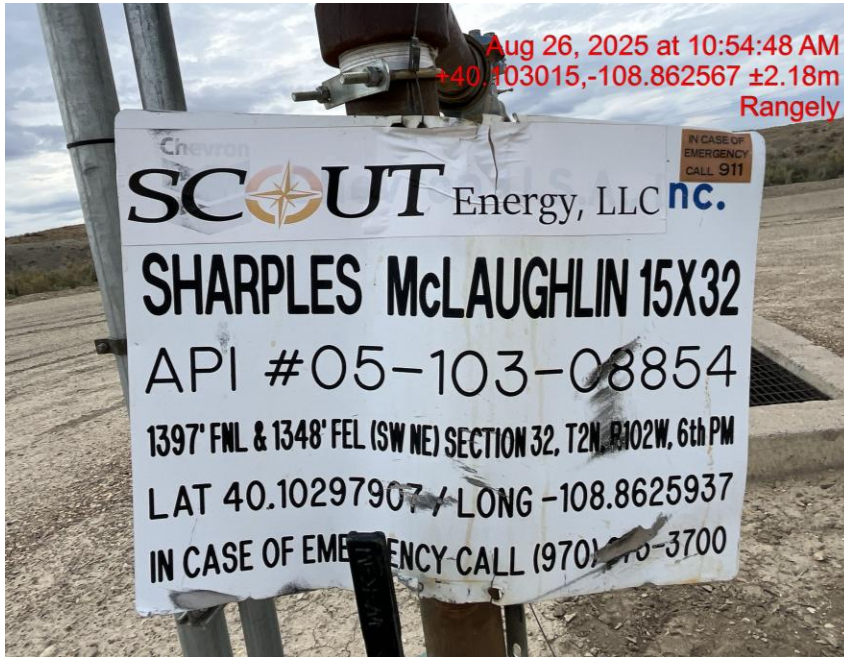
Photo # 2576 Emergency contact number on wellhead sign is not legible/not in compliance with CECMC rules
