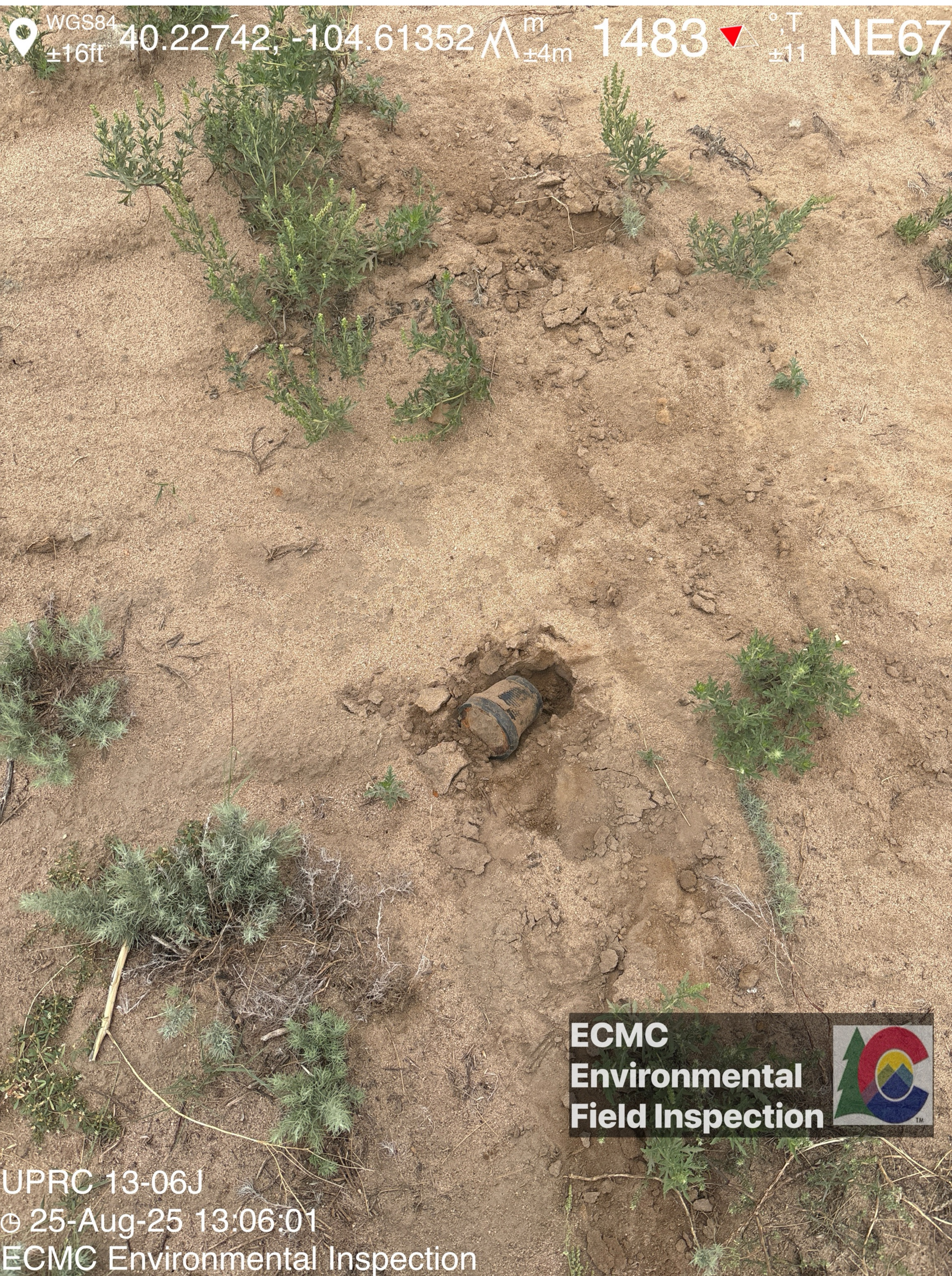
Pieces of trash or E&P waste (pipe fittings) were visible in multiple areas of the location.
